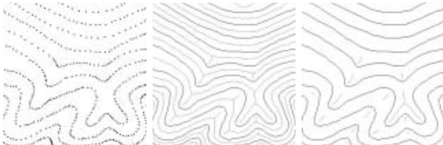
Figure 3. Contours: a) data points; b) crust and skeleton; c) crust and skeleton branches
