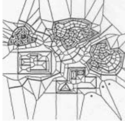
Figure 1 A Voronoi diagram of points and lines.
